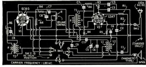
Fig. 1. Schematic circuit of the unit with Sw.2 in the "talk" position. See List of Parts for values.
